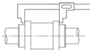
Illustration 4.3.1: Checking the distance between the two half couplings.
